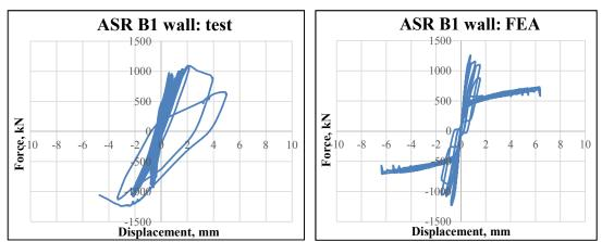
Figure 8. Lateral Force vs. Displacement Curve for ASR B1 wall (after 610 days of accelerated aging)
