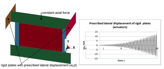
*Figure 2.Outline of FE model and applied loading*
