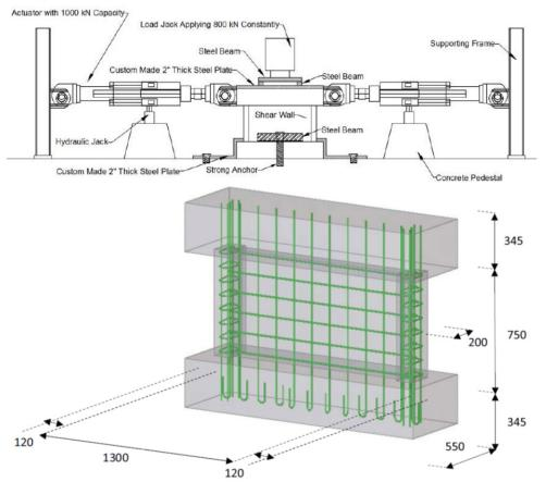
*Figure 1. Test setup [4] and wall geometry. All dimensions are in cm [6]*
