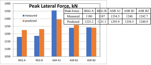
Figure 4 shows predicted and measured Maximum Shear Capacity for all walls.
