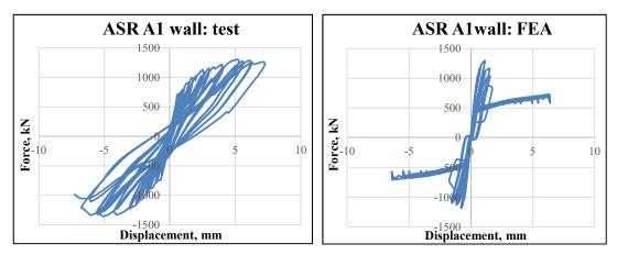
Figure 7. Lateral Force vs. Displacement Curve for ASR A1 wall (after 260 days of accelerated aging)
