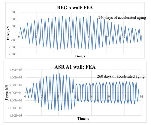
Figure 3. Predicted time histories for the total lateral force for regular (REG A) and ASR A1 walls
